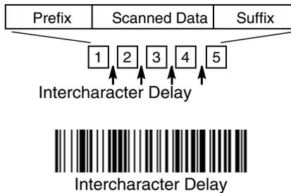
To remove this delay, scan the **Intercharacter Delay** barcode, then set the number of steps to 0. Scan the **Save** barcode using the [Programming Chart](#) inside the back cover of this manual.
