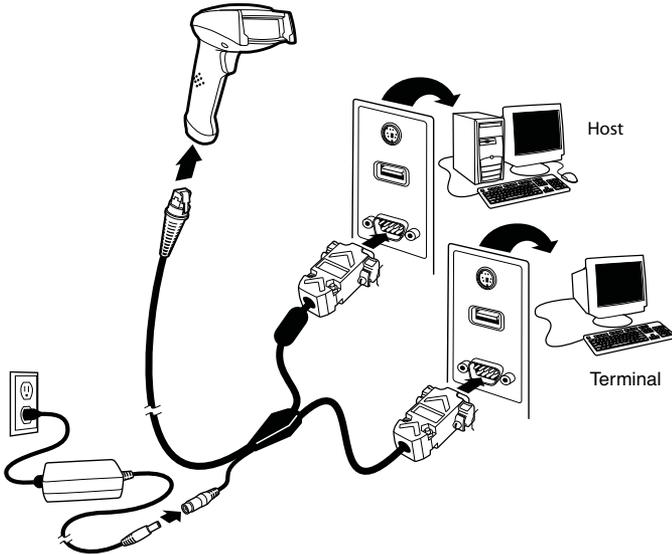
4. Plug the serial connector into the serial port on your computer. Tighten the two screws to secure the connector to the port.
