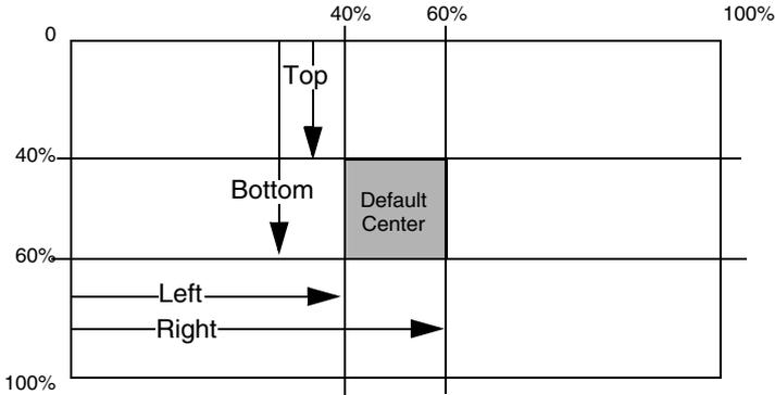
If a barcode is not within the predefined window, it will not be decoded or output by the imager. If centering is turned on by scanning **Centering On**, the imager only reads codes that intersect the centering window you specify using the **Top**, **Bottom**, **Left**, or **Right** barcodes.
